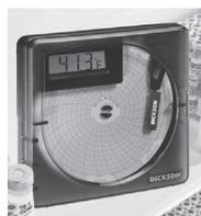
The Dickson Drug Recorder may help organizations ensure compliance with safety and regulatory requirements overseeing temperatures of refrigerators and freezers used in medication storage. The product is small, runs on one AA battery, and measures temperatures in the range of -22°F to +122°F. Functional attributes include an ability to easily print out temperature logs and monitor temperatures during off hours.
