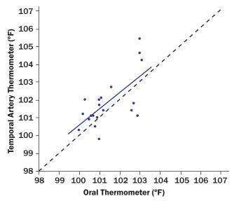
Note. The solid line represents the least-squares regression slope for that data collector. The less scatter of the data points around the line, the greater the equivalence. The dashed line (slope = 1) represents ideal measurement and correspondence of the two instruments.
